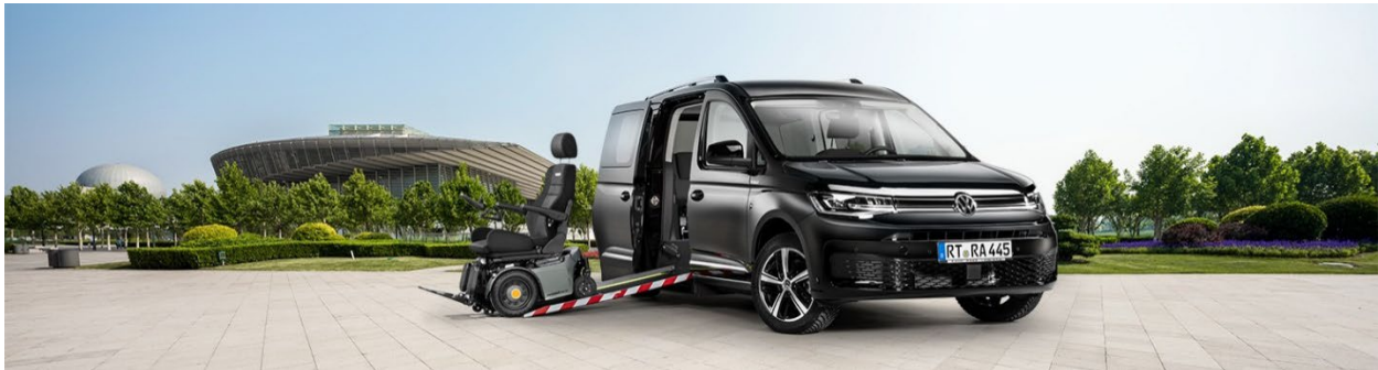
At the touch of a button or remote control, the side door opens, the air suspension lowers the vehicle, and the ramp folds out. Many PARAVAN customers appreciate the side entry solution in the compact VW Caddy 5 Maxi. Photo: PARAVAN
