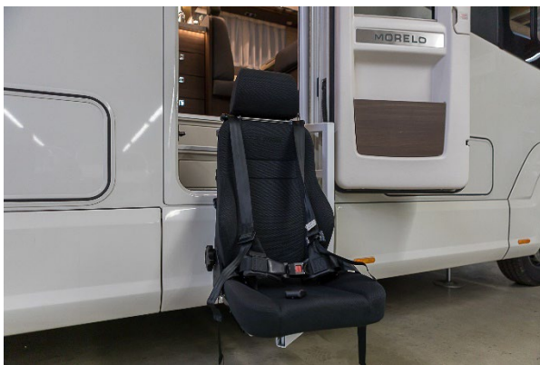
At the touch of a button, people with disabilities can be lifted into the motorhome with the eStep-comfort, photo: PARAVAN
