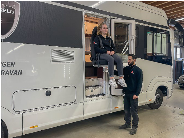
The universal PARAVAN "EStep light" or "EStep comfort" step-on standing lift is the ideal solution for anyone who has difficulty getting into the vehicle but is not necessarily dependent on a wheelchair or is still able to transfer. Photo: PARAVAN
