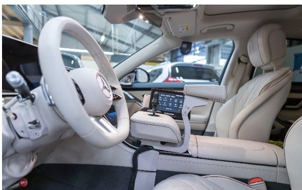
Despite the mechanics, a layman would not even notice that there are struts for the indicators, lights and gear lever on the steering column. Everything has been harmoniously integrated into the vehicle design with great attention to detail. Photo: PARAVAN
