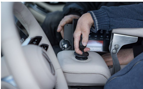
The arm must be positioned comfortably without restricting the freedom of movement to the right and left (steering) or to the front and rear (accelerator and brake). Photo: PARAVAN
