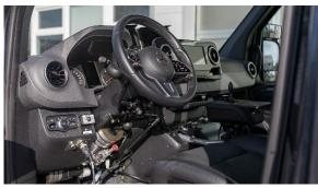
The Mercedes Sprinter of the PARAVAN driving school offers many options and can be converted very quickly as required, from a simple mechanical slope control unit to the Space Drive electronic driving and steering system. Photo: PARAVAN
